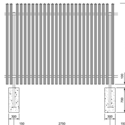
**TYPICAL PALISADE FENCE ELEVATION**
